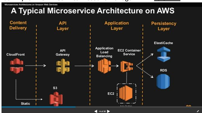
A Typical Microservice Architectur e on AWS S3 CloudFront EC2 Application Load Balancing Static Content Content Delivery API Layer Application Layer Persistency Layer API Gateway EC2 Cont Service Auto Scaling Group DynamoDB
